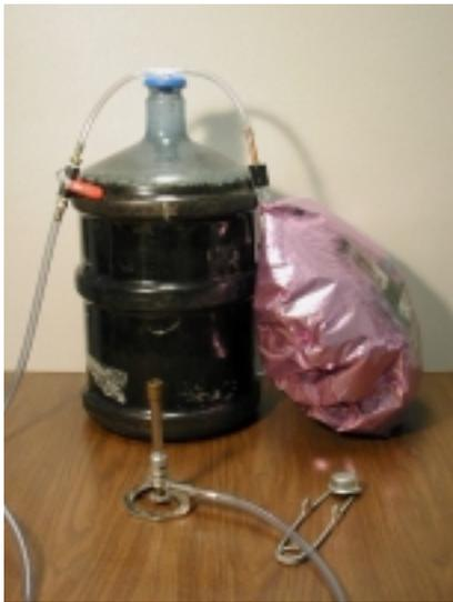
Completed biogas generator.
